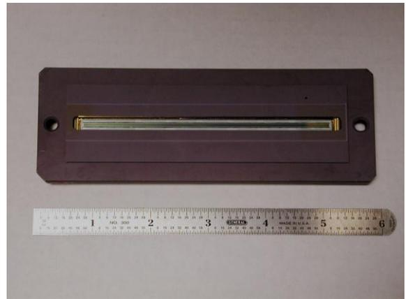
The active imaging area is separated from the eight horizontal output registers by 21 isolation rows. These isolation rows are covered by a metal lightshield to protect them while charge transfers to the output registers. Both the active imaging area and the isolation region utilize 3-phase clocking.
